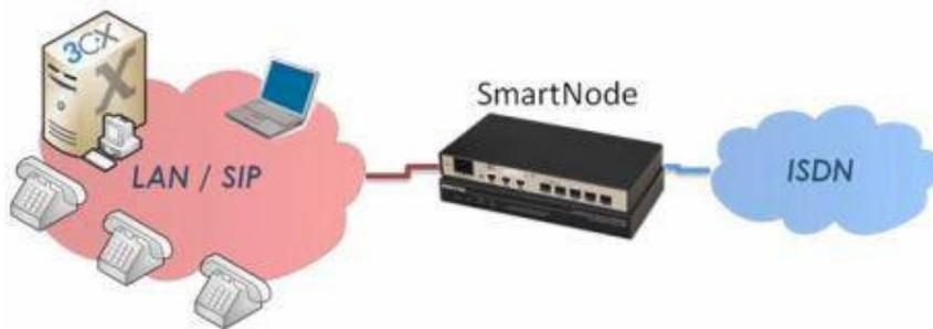
SmartNodes are also widely used to connect to analog PSTN lines or to integrate fax machines and other existing equipment. To make things easy for the end user and system integrator, the 3CX software contains an **integrated SmartNode configuration file generator**. With a few mouse clicks, it generates a full SmartNode configuration file, ready to use and fully interoperable with the system.
