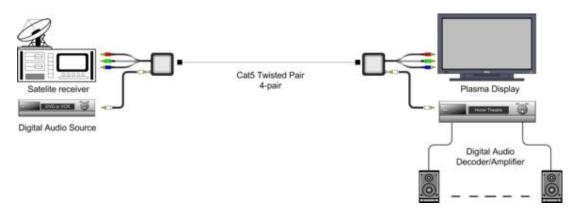
Some DVD players feature up-converter capability that supports HDTV formats. They can also be played out through the structured cabling system as a cost-efficient alternative to the tri-coax component cables.
